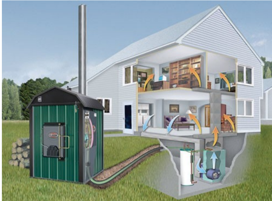
Figure 17: Operational Diagram of a Wood Furnace (Central Boiler, 2008)
