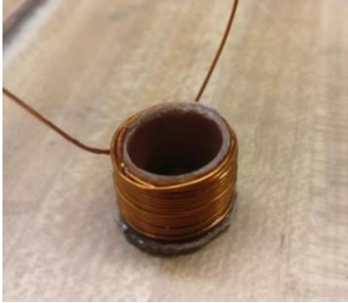
Figure 14. Fabricated solenoid coil with R/L = 1 .
