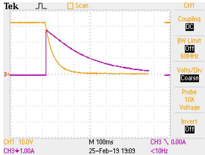
Figure 21. Oscilloscope transient response of LRC circuit from circuit testing.
