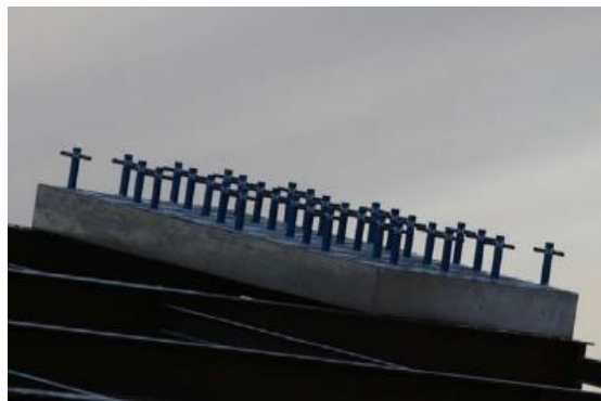
Figure 4.1.9 A panel of crossed dipoles (32 antennas)
