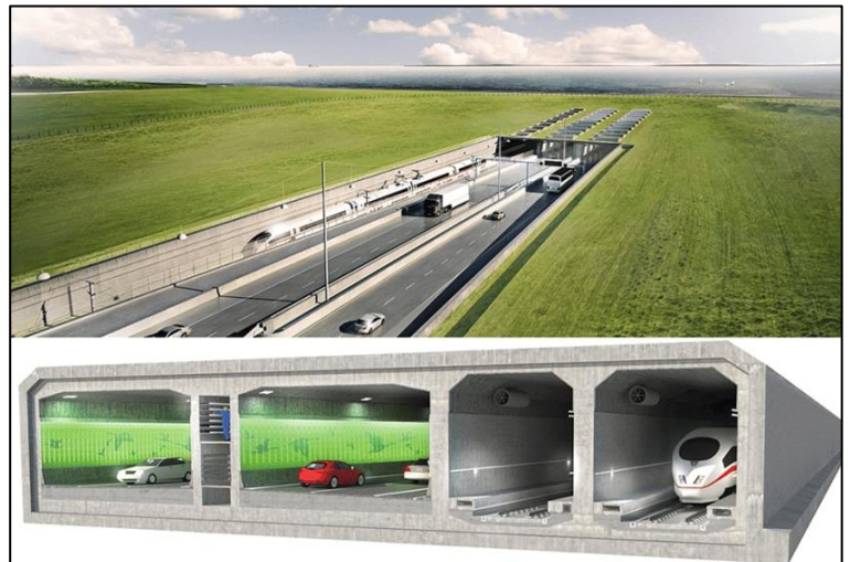
Figure 18: Design of the immerse tunnel between Danish Island of Lolland with Fehmarn of Germany (Fehmarn, (n.d.)).
