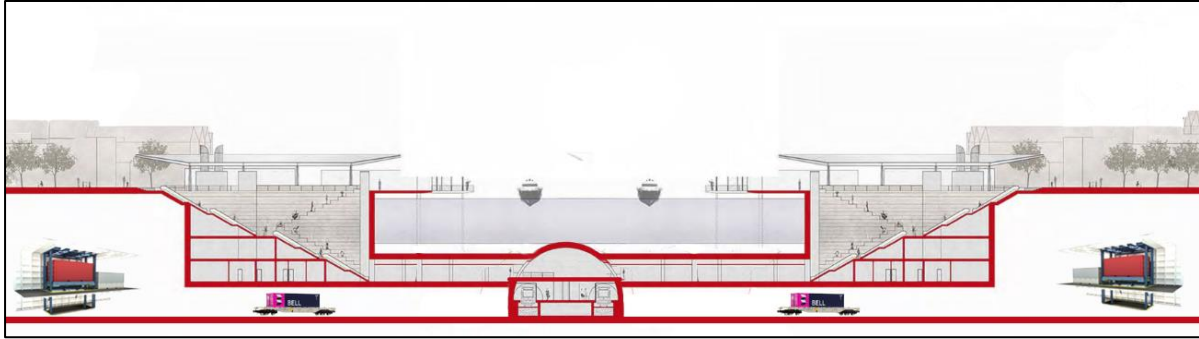
Figure 39: Design of the new station with two pedestrian connections. Adapted from the original design of the thesis “Una Metropolitana Sub-lagunare per Venezia” (Villalobos 2022).
