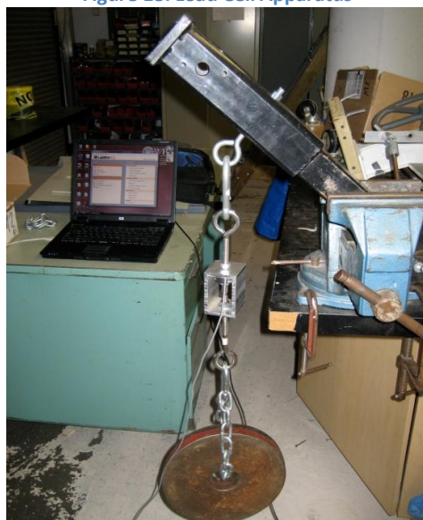
Figure 19: Calibration of Final Load Cell Apparatus
