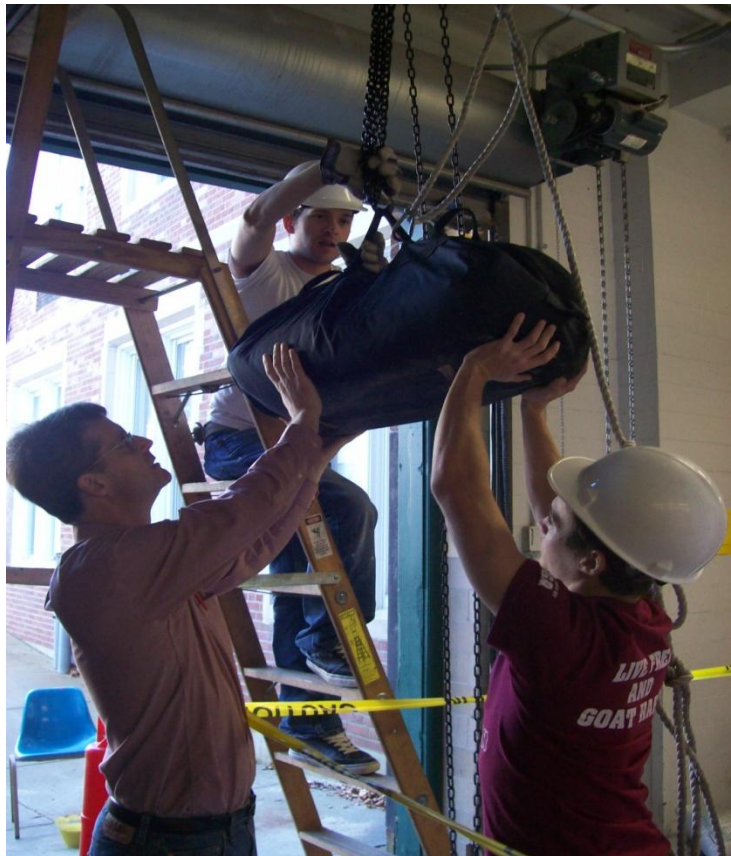
Figure 23: Kite System Testing Using Sandbags to Simulate Kite Tension
