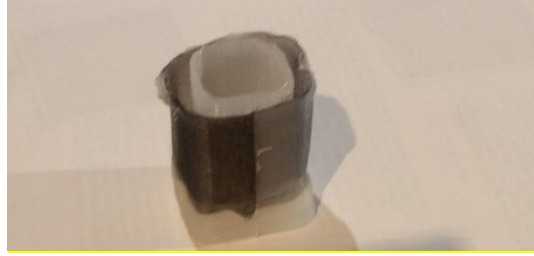
Figure 82: Successful Attempt of Molded Silicone Rectangular Toroid
