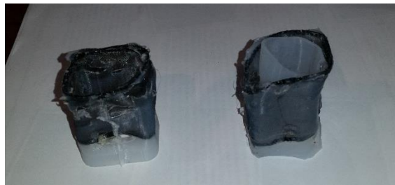
Figure 81: Initial Attempts of Molded Silicone Rectangular Toroids
