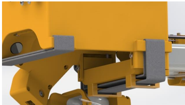
Figure 13: Tube input from pal module and use of HERO Glove's strap
