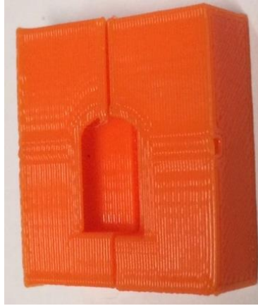
Figure 36: Robot Grip Force sensor silicone mold
