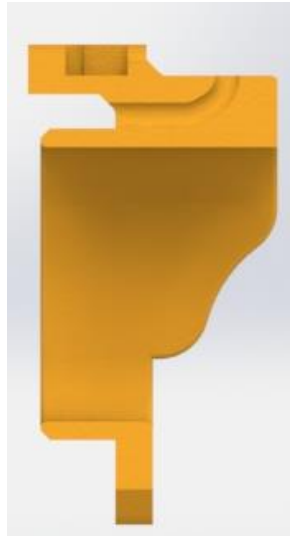
Figure 15: Finger joint actuator input tube channel
