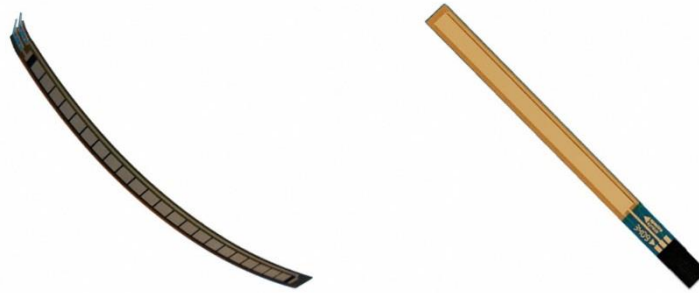
Figure 20: Resistive flex sensors that we have tested
