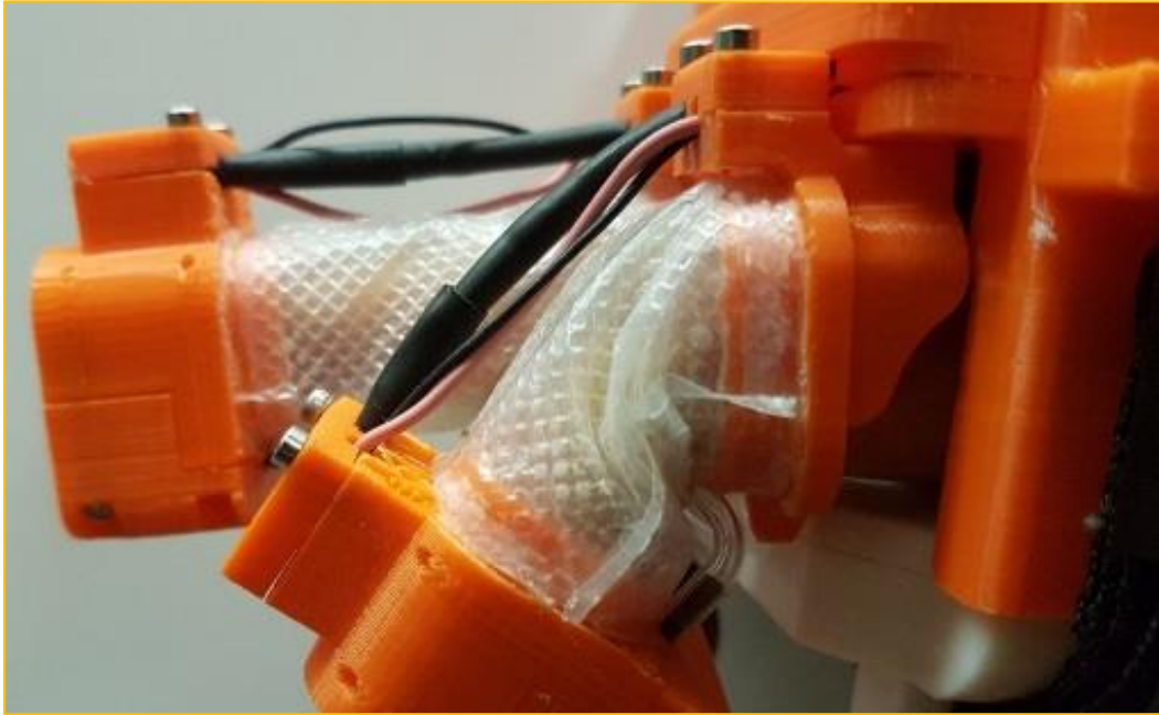
Figure 22: Light-based curvature sensor mounted on finger module
