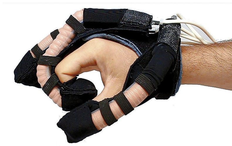
Figure 4: Soft robotic glove using soft pneumatic actuators for rehabilitation
