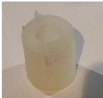
Figure 80: Successful Attempt of Molded Silicone Cylindrical Toroid
