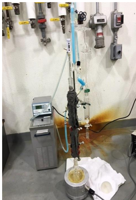
Figure 11: Packed Column Batch Distillation Tower Used in Lab
