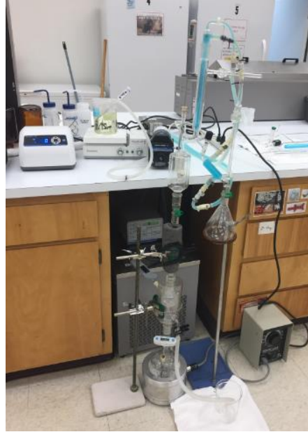
Figure 31: Valve-Tray Steam Stripper Used for Fusel Oil Steam Stripping
