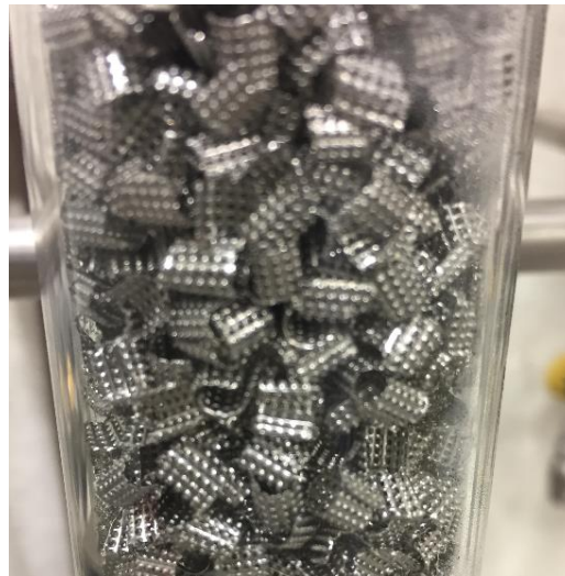
Figure 10: Pro-Pak® Packing used in Batch Still
