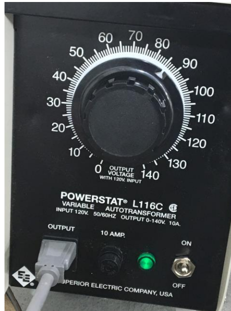
Figure 6: Power Stat Used for Controlling the Heating of the Still
